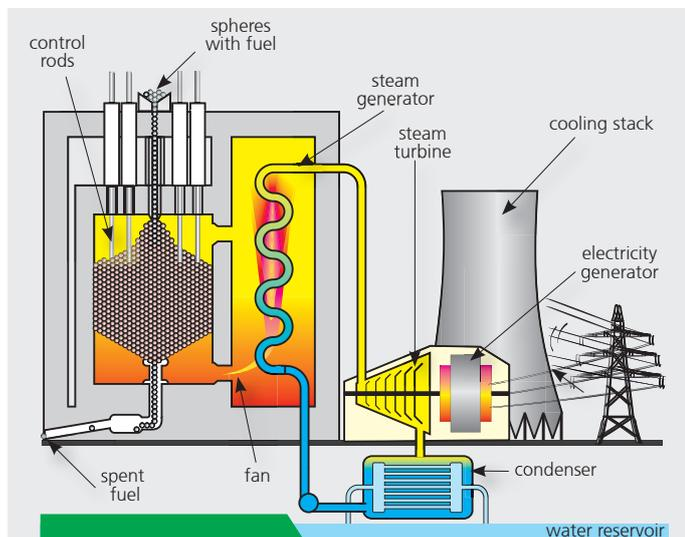
**Layout of a high-temperature reactor NPP**
