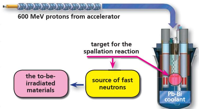
**Reactor output 50-100 MWth in subcritical state, around 100 MWth in critical state**
