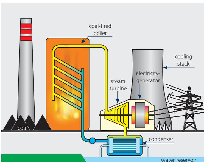
Layout of a coal-fired power plant
