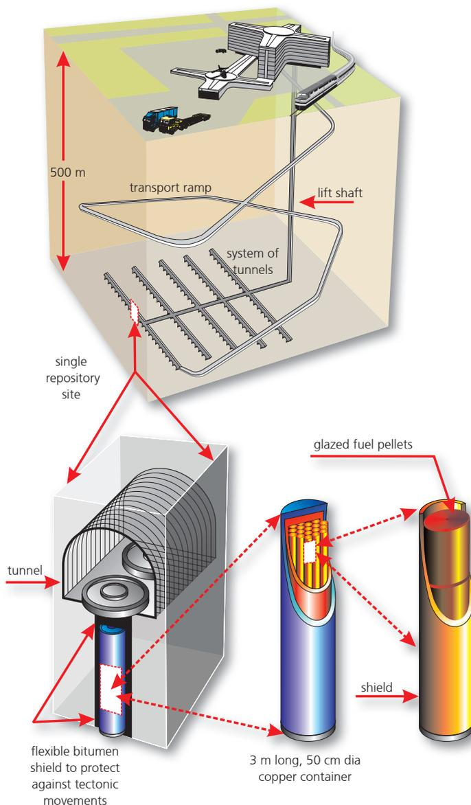
**Layout of a typical nuclear waste underground repository**
