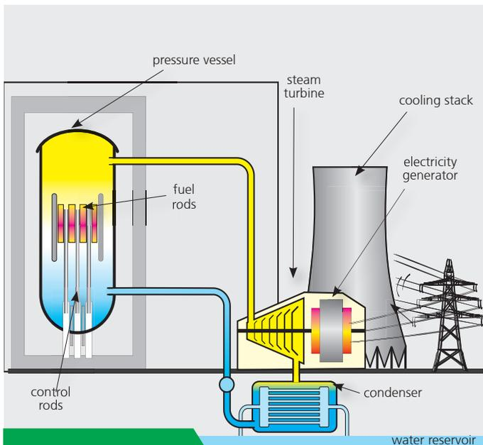
**Layout of Boiling Water Reactor NPP**
