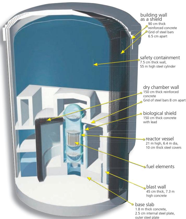
**Multiple safety barriers built into nuclear reactors (a typical BWR reactor is shown as an example)**
