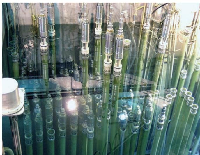
**Spent fuel immersed in water of the MARIA reactor storage tank**
