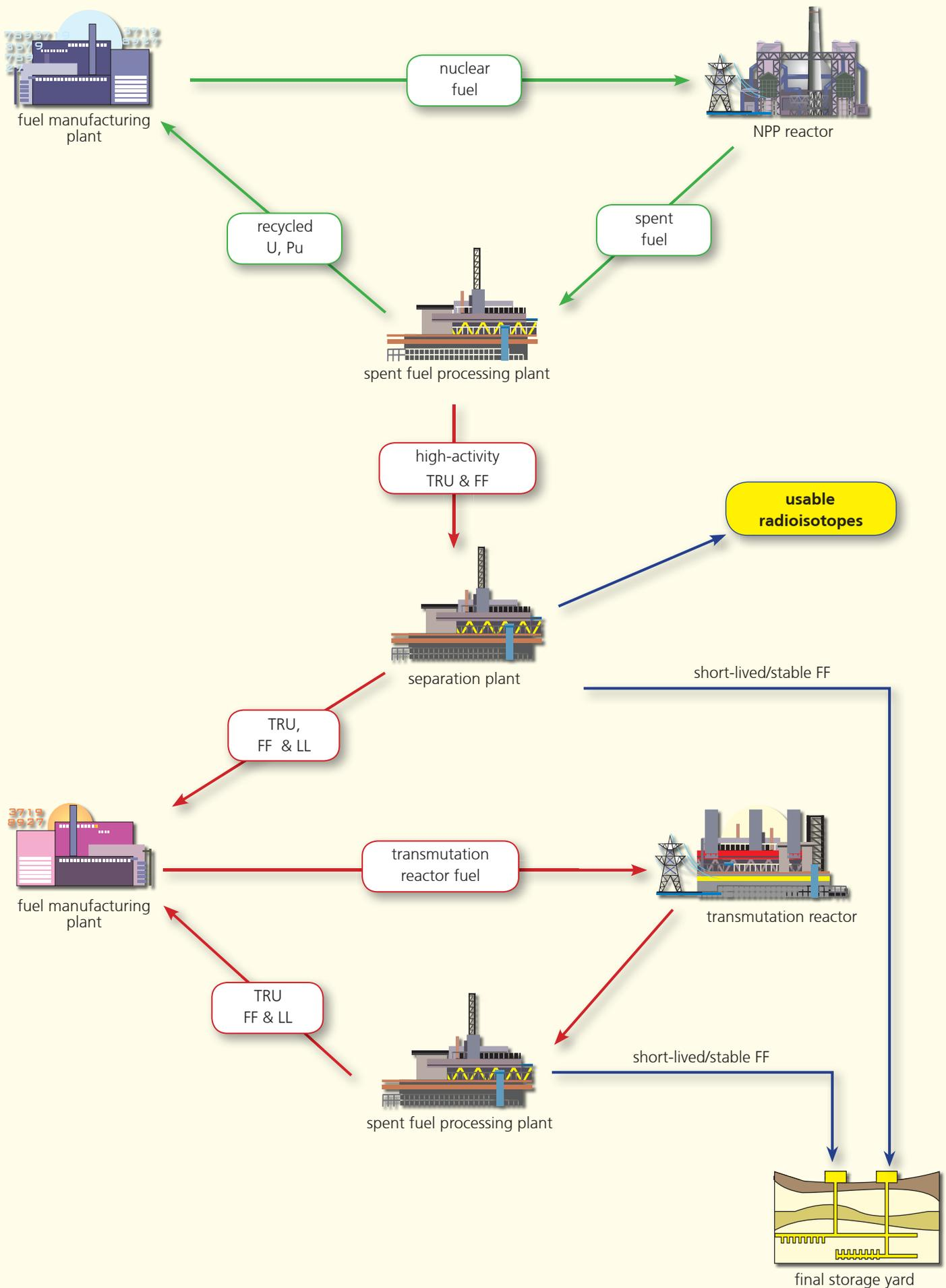
**Block diagram of a possible closed fuel cycle**
