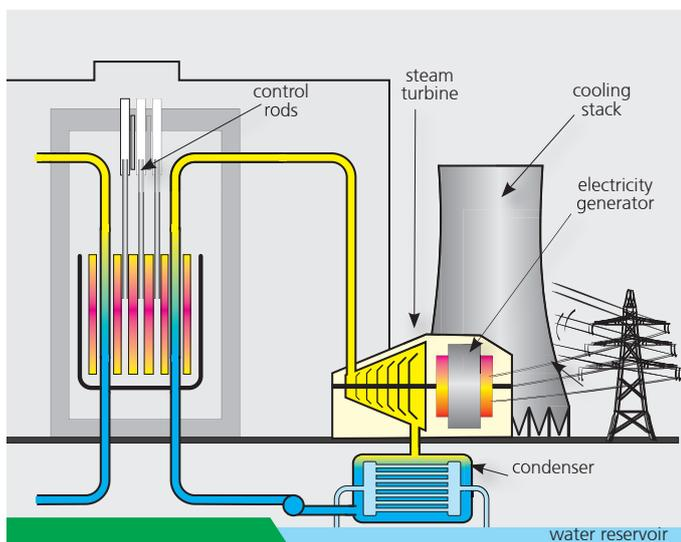
**Layout of a RBMK reactor NPP**
