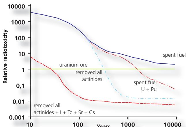
**Influence of spent fuel processing on radiotoxicity of highly active waste produced in nuclear power reactors** (after G.J. van Tuyle et al., Nucl. Tech. 101 (1993) 1)
