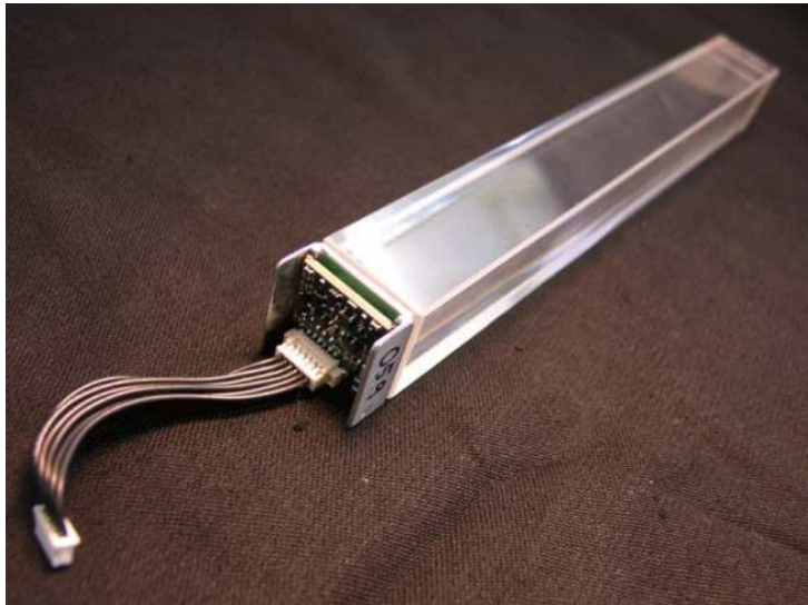
Figure 2.8: The avalanche photodiode connected to the scintillation cell.
