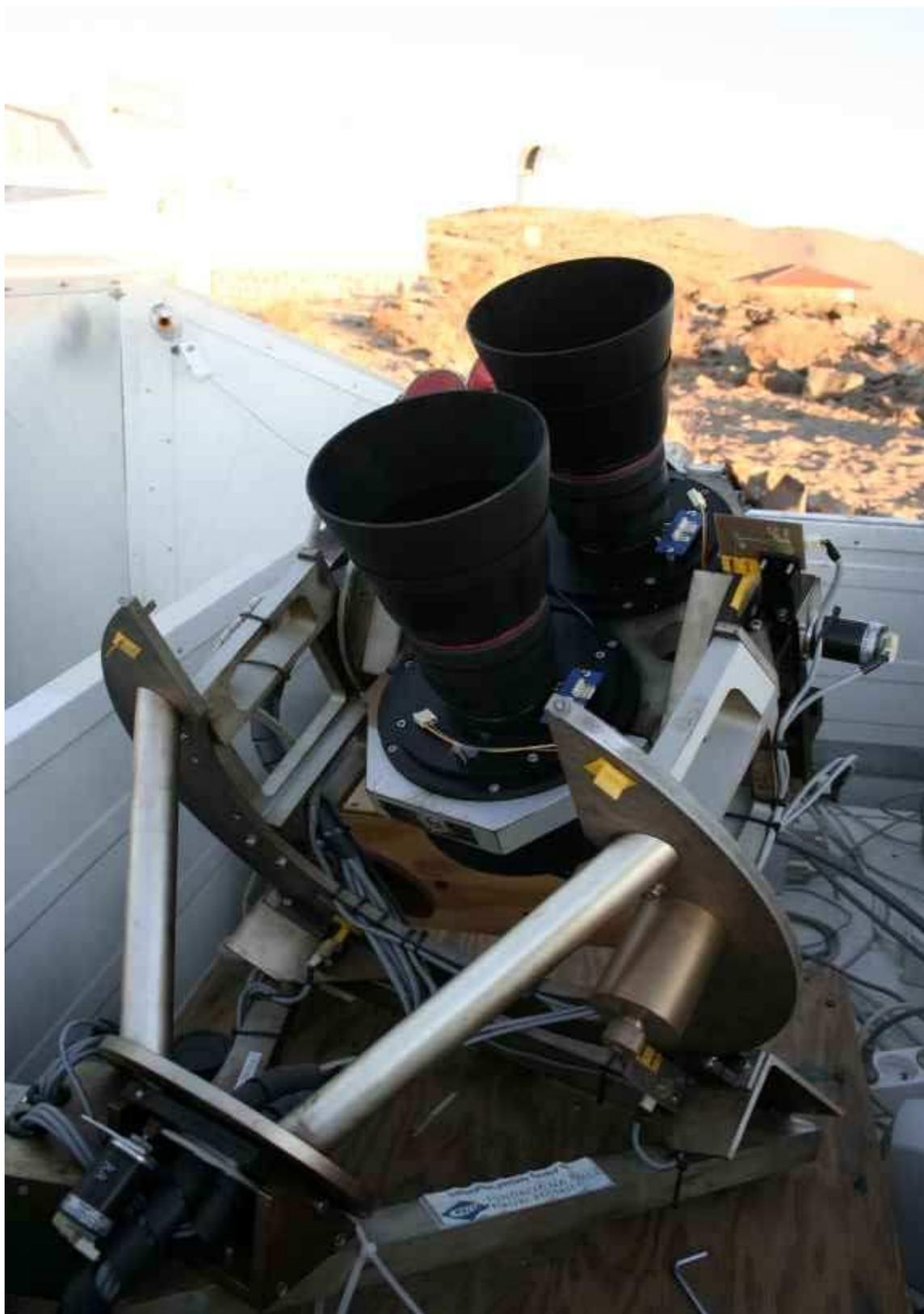
Figure 2.1: The prototype in LCO, two cameras on a single mount in the ASAS dome
