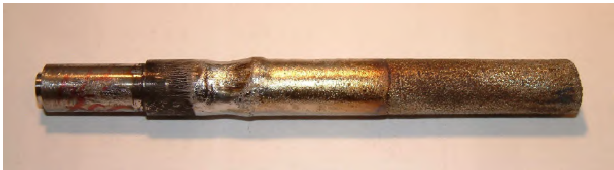
Figure 10. Erosion traces of the IPD accelerator internal electrode.
