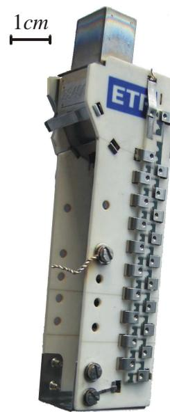
Figure 36: Photo of a DDEM type AF180H detector.
