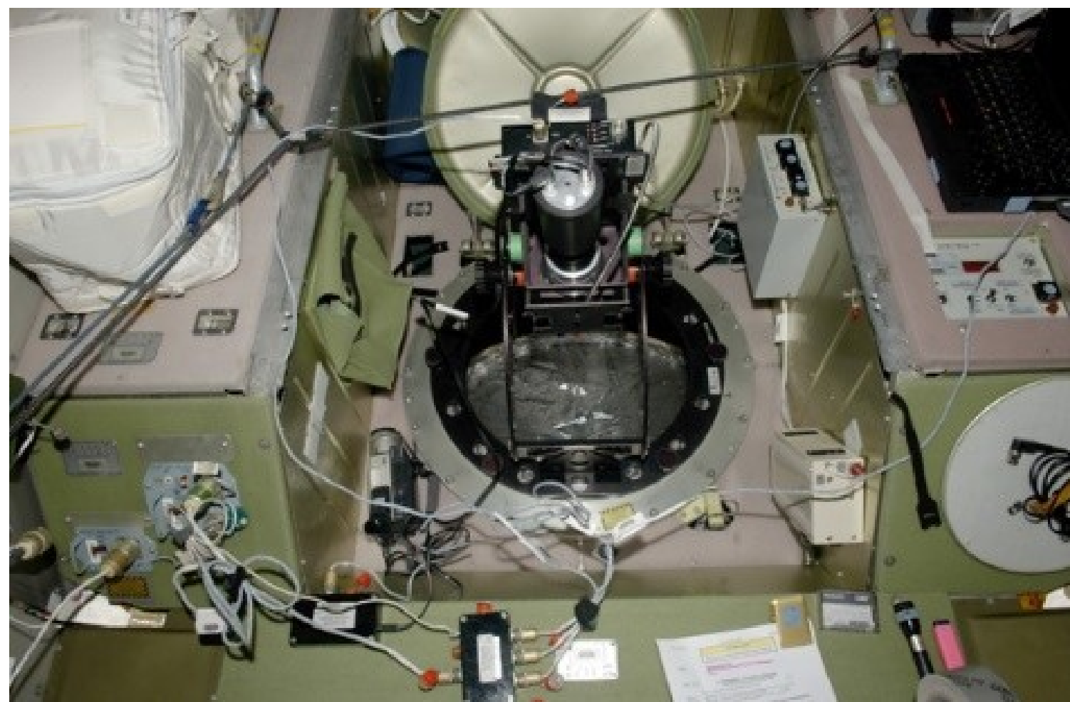
5 Position of UV transparent window in ISS
