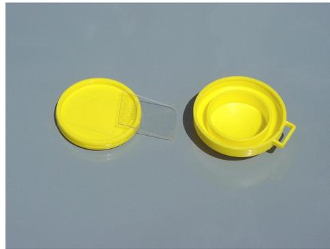
Fig. 1. Opened NRPB-type dosimetric cassette with a Cr-39 detector.
