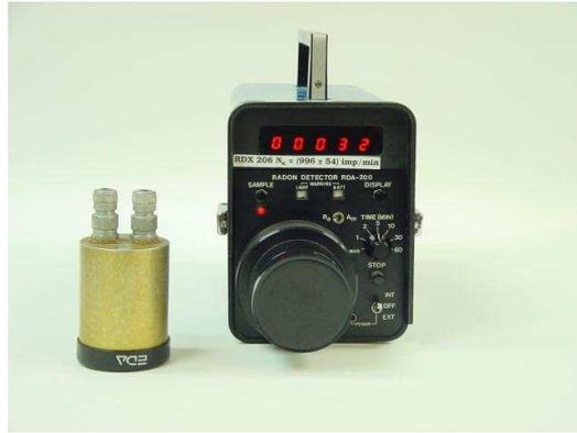
Fig. 2. RDA-200 gauge by Pylon (Canada)
