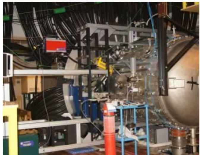
Fig. 26 FNYM (inside the yellow frame) mounted on the vacuum vessel wall of the PF-1000
