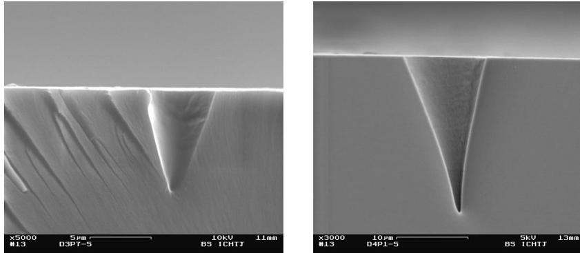
Rys. 4. Sample of pictures presented craters of alpha particles of energy 5.5 MeV.
