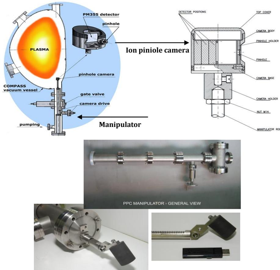
Fig. 21. Specially designed ion pinhole camera dedicated for COMPASS tokamak.
