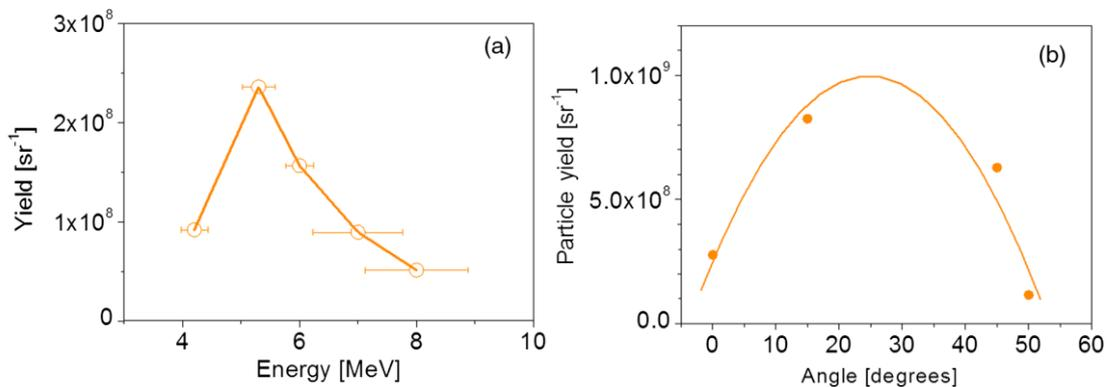
Rys. 10. (a) Alpha-particle energy distribution obtained from PM-355 analysis using detectors shielded with different Al filter thicknesses (6–20  $\mu$ m) and placed at an angle of about 45° with respect to the laser-incident direction in the same laser shot. (b) Alpha particle angular distribution obtained from PM-355 analysis using detectors placed at different angles with respect to the laser-incident direction in the same laser shot.
