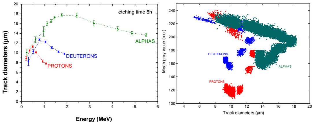
Fig. 1. Track diameters presented vs particle energy. Two-dimensional distribution of the mean grey level values as a function of track diameter.
