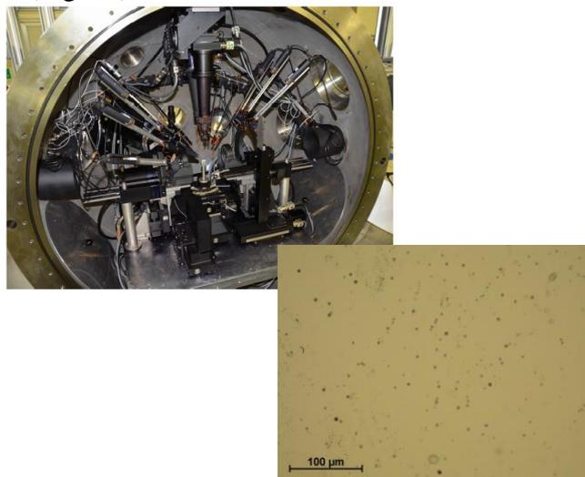
Fig. 12. Example photos of the ABC laser system and image of craters produced by protons.
