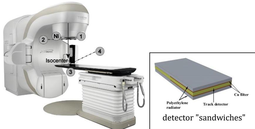
Fig. 19. Scheme of the placement of detector “sandwiches” around the accelerator head and in the patient plane. Samples #1 and “Ni” were located near the accelerator head. Sample #2 was located about 100 cm from the conversion target, samples #3 and #4 were placed in the patient plane.
