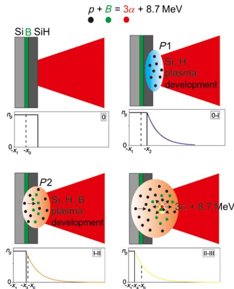
Fig. 7. Laser-target, laser-plasma, and proton-boron interactions in the 2-ns range before the maximum laser intensity.
