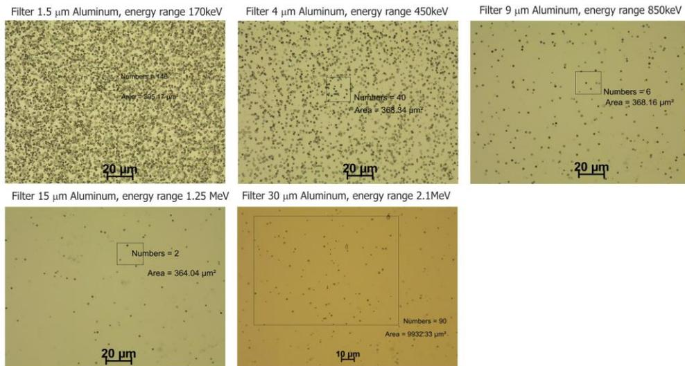
Fig. 14. Ion Track Detectors covered by different filters and irradiated by a stream of protons from several laser pulses.
