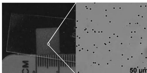
Fig. 16. Picture of ion beams profiles measured by the CR-39/PM-355 detector.
