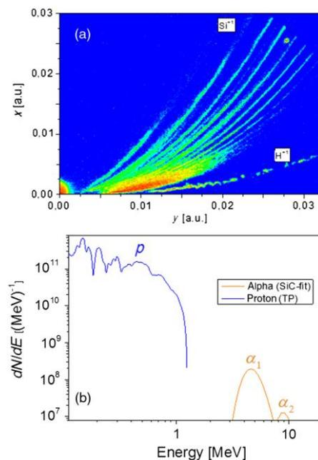
Fig. 11. (a) Typical TP spectrometer images showing the presence of backward-accelerated protons and heavier plasma ions. The corresponding proton-energy distribution and the comparison with the alpha-particle one (obtained by fitting the TOF spectrum) are shown in (b).
