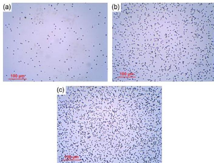
Rys. 17. The results of the PM-355 track detectors irradiated with: (a) 0.05 Gy, (b) 0.5 Gy, (c) 1 Gy of  $^{12}\text{C}$  ions – results after 2 h of etching.
