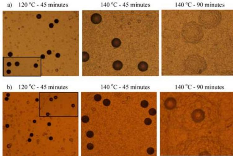
Fig. 2. Sample photos of tracks observed in PM-355 detector samples which were etched for 5 h. The tracks were induced by: (a) 3.0 MeV  $\alpha$  particles, (b) 5.0 MeV  $\alpha$  particles.
