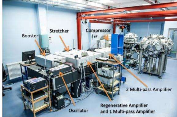
Fig. 13. IPPLM Laser Laboratory and important parts of Femto-Second Laser system.
