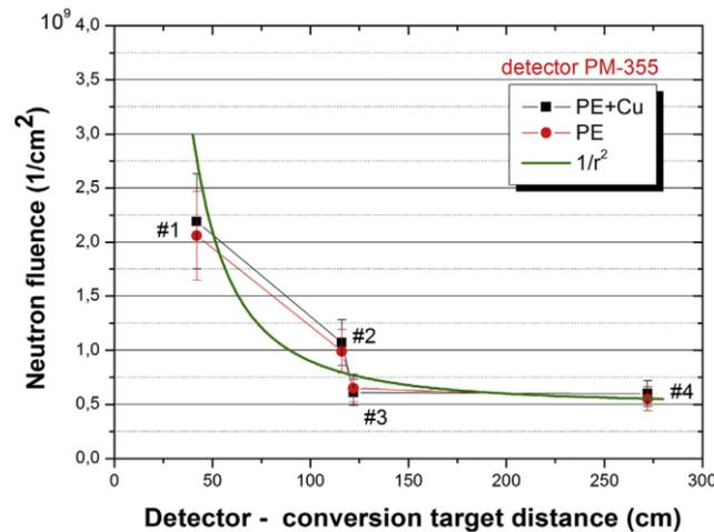
Fig. 20. Total neutron fluences recorded by the samples versus the distance from the accelerator conversion target. Detector numbers correspond to the locations shown in Fig. 19.
