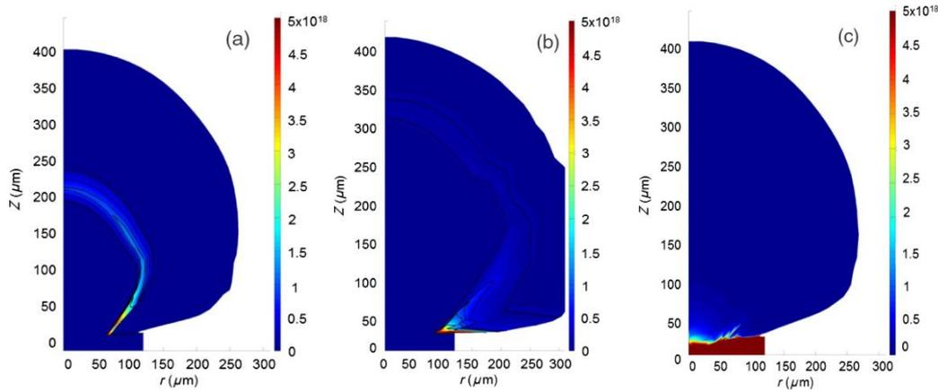
Fig. 8. 2D PALE hydrodynamic simulations of the boron plasma expansion after the action of the laser pulse (in the range 1–1.85 ns) for (a) the B layer implanted in the SiH substrate, (b) the B layer deposited on the SiH substrate, and (c) the B layer diffused in the SiH substrate. The gradients scale on the right-hand side shows the B-plasma density.
