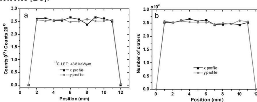
Fig. 15. Profiles of ion beams measured using: a – Si detector; b – PM-355 detector.
