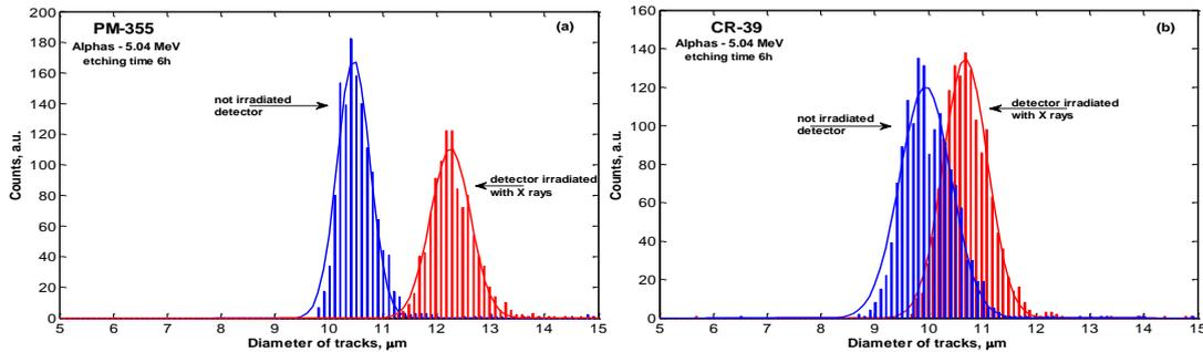
Fig. 5. Histograms of crater diameters as measured in PM-355 and CR-39 detector samples which were first irradiated with 5.04 MeV alpha particles and then exposed to X ray radiation delivered by an X ray tube. The blue curves represent histograms of crater diameters measured in the samples which were not exposed to the X ray radiation.
