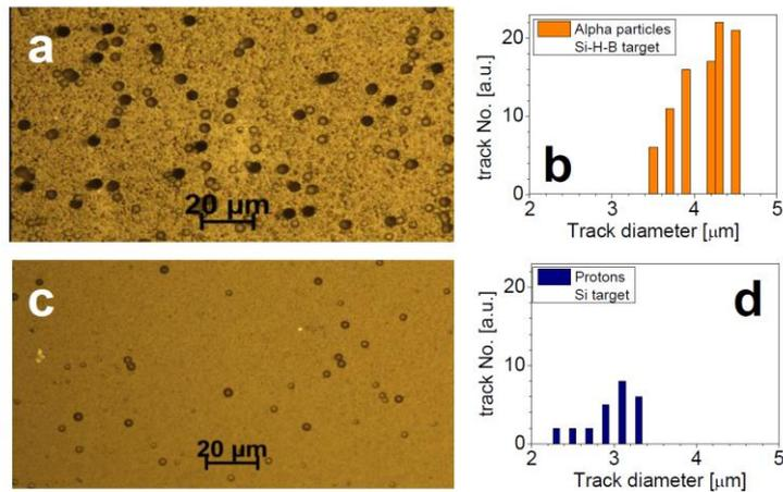
Fig. 9. Examples of craters produced by incident protons (small light craters) and alpha particles (large black craters) for (a) the Si-H-B target and (b) the corresponding histograms of particle crater diameters. (c) Craters produced by incident protons for the Si target and (d) corresponding histograms of particle crater diameters.
