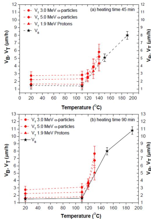
Rys. 3. The bulk etch rates  $V_B$  of PM-355 detector material and track etch rate values  $V_T$  as determined for craters induced by protons and  $\alpha$  particles. The detector samples were etched for 5 h and the diagrams are presented versus the heating temperature for two different heating times: (a) 45 min and (b) 90 min.
