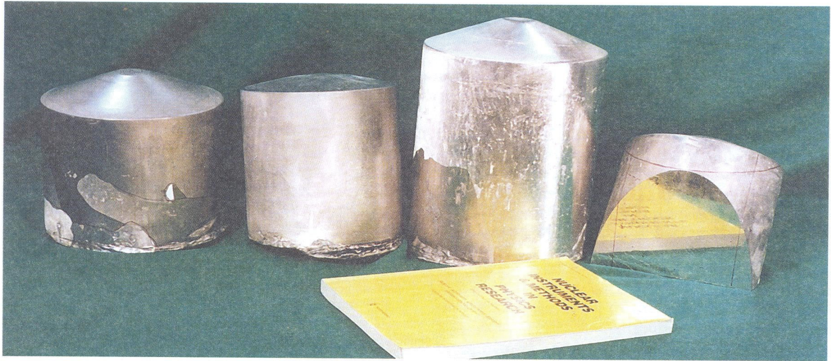
Fig. 1. Bismuth single crystals of diameters 17 cm and 19 cm obtained by modified method.
